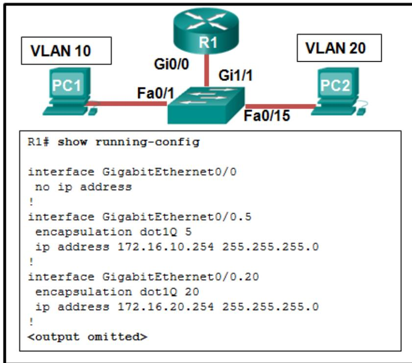
Refer to the exhibit. A network administrator is verifying the configuration of inter-VLAN routing. Users complain that PC2 cannot communicate with PC1. Based on the output, what is the possible cause of the problem?
