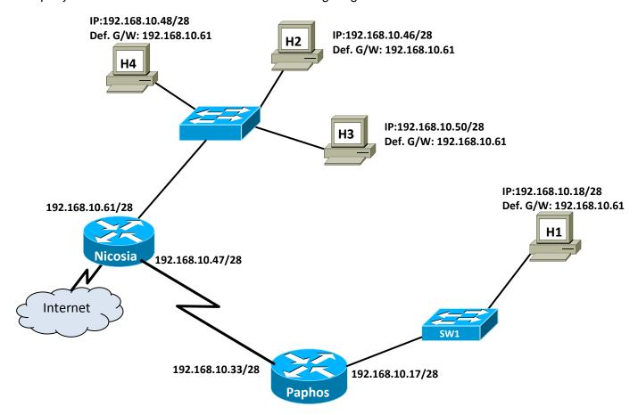
The network technician made **four mistakes** in the network configuration. In the table below specify the host name, the mistake, the reason it is wrong and a way to correct it.
