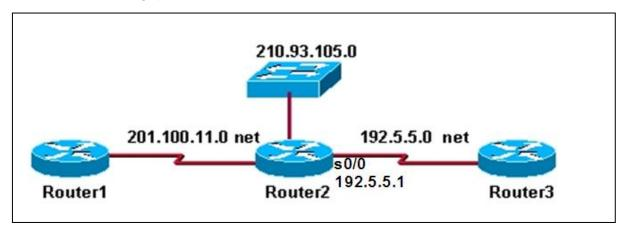
(a) Give the necessary commands for configuring and activating the serial interface S0/0 of router2 (192.5.5.1). Assume that the router is initially in privileged mode.
