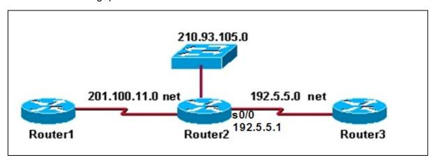
a. Give the necessary commands for configuring and activating the serial interface S0/0 of router2 (192.5.5.1). Assume that the router is initially in privileged mode. (4 pts)
