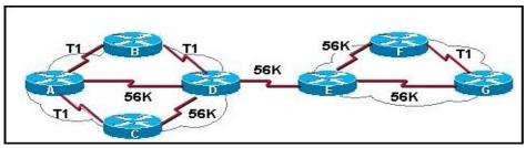
Refer to the exhibit. Assuming default metrics are used and the network is fully converged, which path will RIP use to send a packet from Router A to Router F? (Choose one.)
