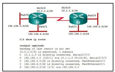
Refer to the exhibit. A ping from R1 to 10.1.1.2 is successful, but a ping from R1 to any address in the 192.168.2.0 network fails. What is the cause of this problem?
